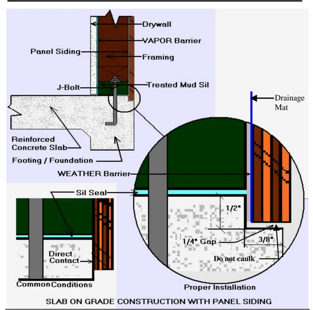
For siding in slab on grade construction to be successful, moisture migration from the concrete to the siding must be eliminated. The slab should be insulated and have a vapor barrier in place. Direct contact between siding and concrete must be avoided. To achieve the required clearance between siding and grade, the height of the slab must be at least 8" above finished grade.
